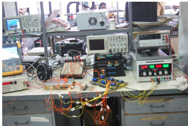
Fig. 9: Experimental Setup of two legged inverter (3-level configuration)
